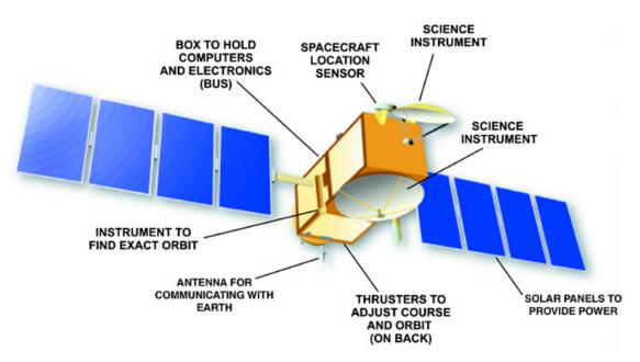
This is the Jason-1 spacecraft. It will be launched early in 2001. It will orbit Earth and study the oceans. It will join its older sibling, the TOPEX/Poseidon spacecraft. TOPEX/Poseidon has been studying the oceans since 1992.
